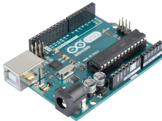
Figure 6. Basic Arduino Set
